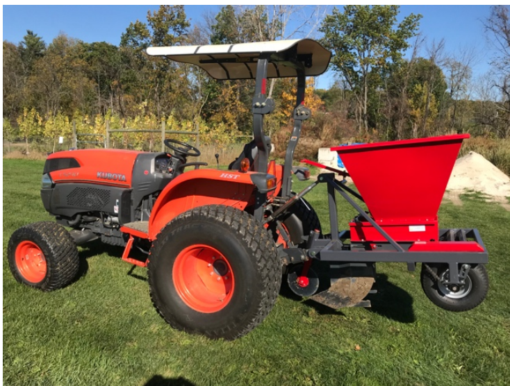
The Geerlings planter (0.5 meter width) on our 45 HP tractor with turf tires. 7583
